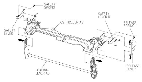
Fig.35 DISASSEMBLY OF THE CASSETTE HOLDER ASS'Y
